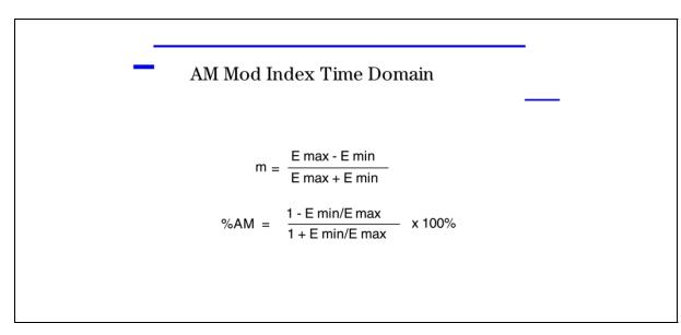
The first formula can be used to calculate m, just like an oscilloscope. However, use the second formula when using the spectrum analyzer's relative markers. Relative markers in linear mode show the ratio. For example, if the relative marker reads "0.1x", this means that the lower signal is "0.1 times" or 10% of voltage of the higher signal.
