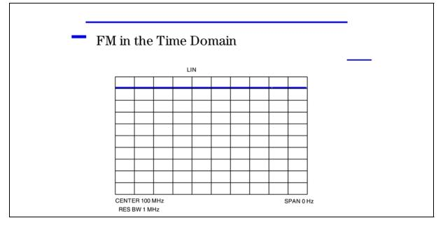
When displayed in the swept-tuned frequency domain, narrowband FM looks just like AM. However, if we open the resolution bandwidth, FM becomes a line on the display, since there are no amplitude variations.
