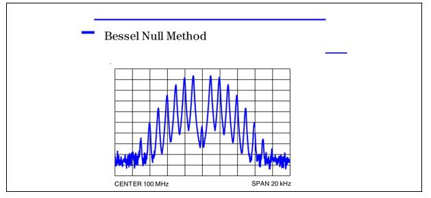
The Bessel function tells us the carrier and sideband amplitudes are a function of m. The carrier component  $J_0$  and the various sidebands  $J_N$  go to zero amplitude at specific values of  $\beta$ . For example, the carrier component achieves a "Bessel null" at precisely  $\beta = 2.4048$ .
