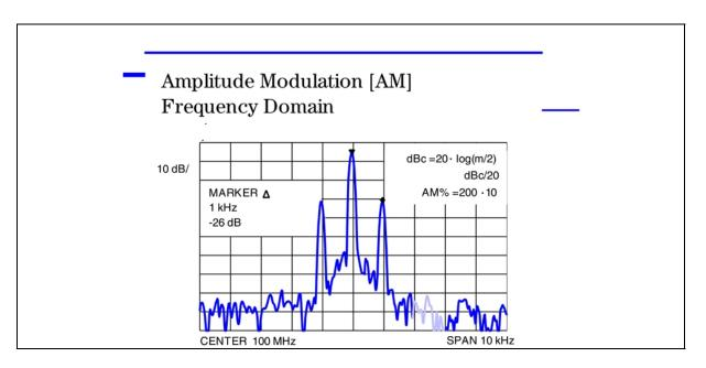
For 100% AM, the sidebands are each 1/2 the amplitude of the carrier or -6 dBc; for 10% AM, the sidebands are 1/10 as large as in the 100% AM case or -26 dBc; for 1% AM the sidebands are -46 dBc, and so on. Hence:  $AM\% = 200 \times 10^{-(\Delta dB20)}$
