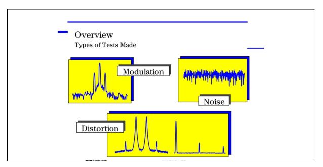
The most common measurements made using a spectrum analyzer are: modulation, distortion, and noise.
